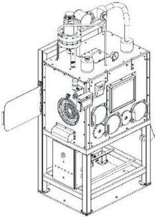
Aquila Nuclear Engineering Ltd was engaged to design and manufacture a shielded containment that could operate as a glovebox in normal conditions, but if a higher radioactive activity sample is received, the cell can be remotely operated using tongs.
