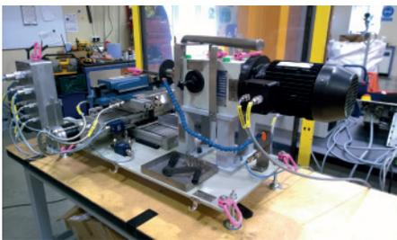
Aquila reviewed the detailed specification supplied by NNL and developed a Remotely Operated Diamond Saw which was simple, practical and cost effective. Careful selection and adaptation of Commercial off the Shelf (COTS) equipment kept much of the machine operation manual. This
